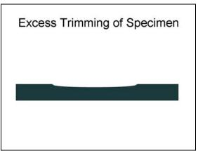
A glass base plate can be used to observe the bottom of the specimen to ensure it has remained in contact with the base, or a light tap on the top of the specimen with a gloved finger treated with a contact release agent. If the specimen has pulled away from the bottom of the plate and material has unintentionally been trimmed from the specimen, a slight trough will be observed.
