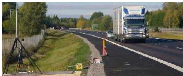
Figure 10. SPB in situ measurement
