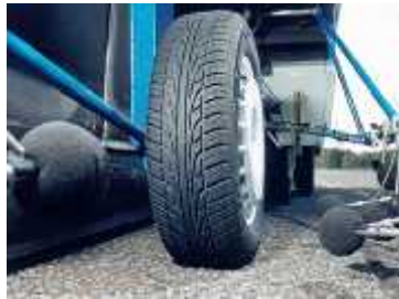
Figure 5. Set of microphones near the tire for the measure with the CPX method
