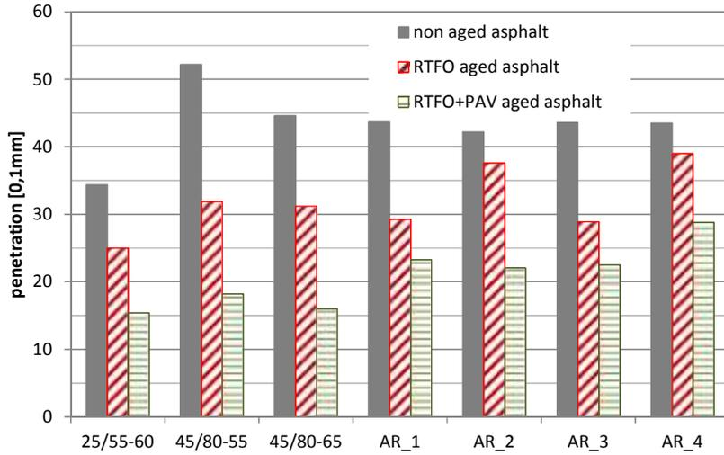
**Figure 1.** Penetration of asphalt rubber and polymer modified bitumen at 25 °C
