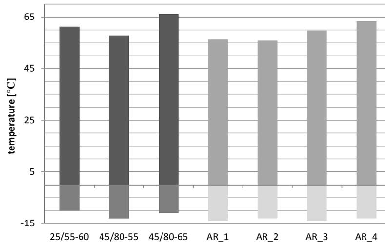
**Figure 4.** Temperature plasticity range of asphalt rubber and polymer modified bitumen.
