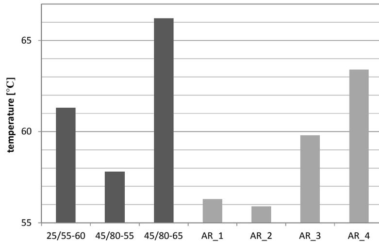
**Figure 2.** Softening point by R&B test of asphalt rubber and polymer modified bitumen
