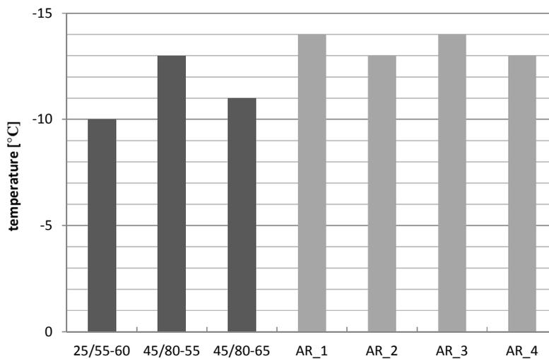
**Figure 3.** *The Fraass breaking point of asphalt rubber and polymer modified bitumen*
