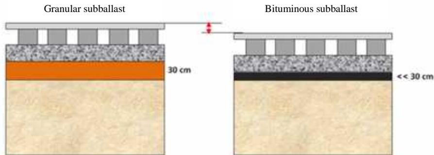
**Figure 3.** Thickness reduction due to higher bearing capacity of bituminous subballast layer
