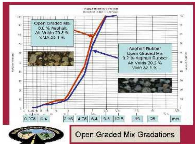
Figure 9. Open Graded Mix and ARFC gradations
