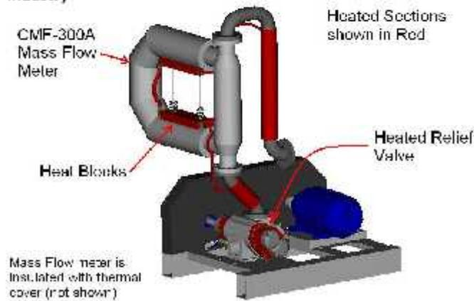
Figure 15. Mass Flow Meter [Motion, 2011]
