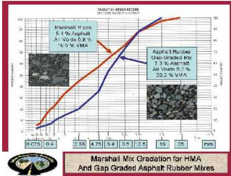
Figure 8. Marshall Mix HMA and ARAC gradations
