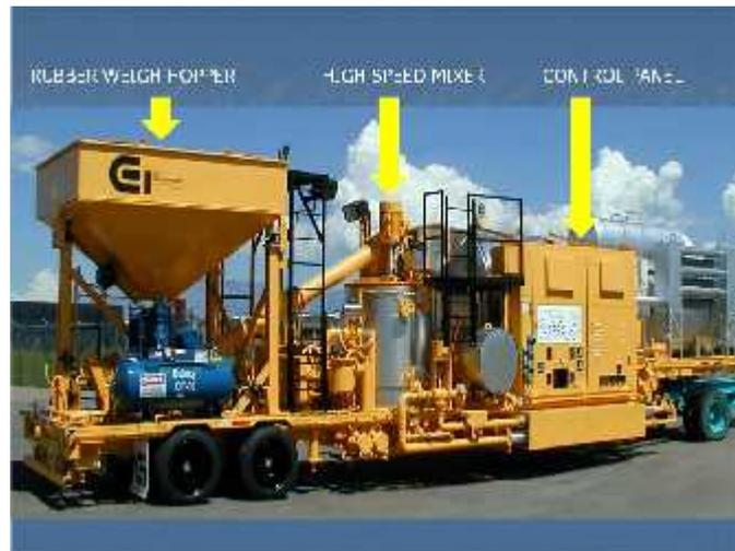
**Figure 11.** Example Ground Tire Rubber and Asphalt Blender Unit
