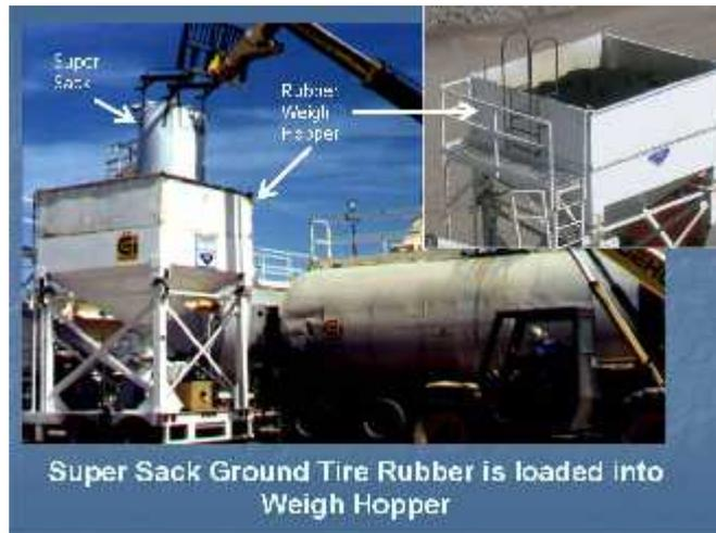
**Figure 10.** Loading Ground Tire Rubber into Weigh Hopper
