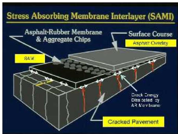
**Figure 7.** *Asphalt-rubber Stress Absorbing Membrane Interlayer (SAMI)*
