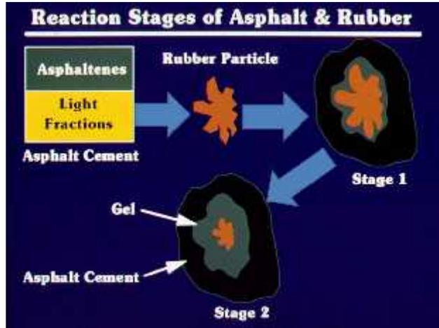
**Figure 2.** Asphalt-rubber reaction/blending process
