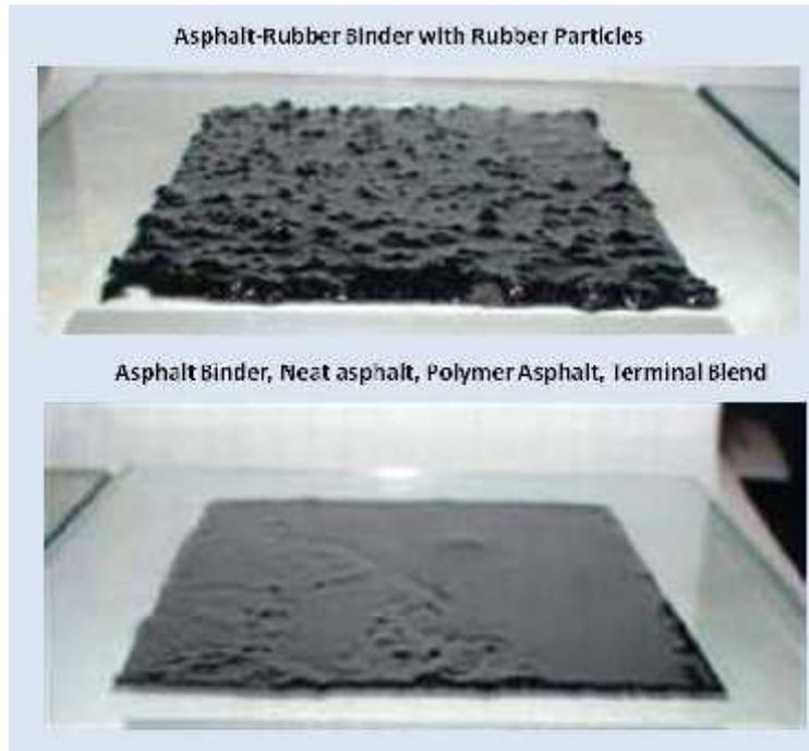
**Figure 1.** Asphalt-rubber with rubber particles compared to other forms of asphalt binder
