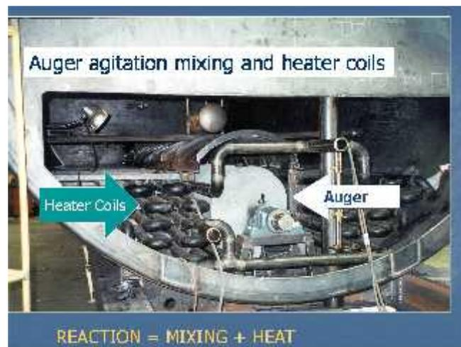
**Figure 13.** Example Blend Tank with Heat and Agitation
