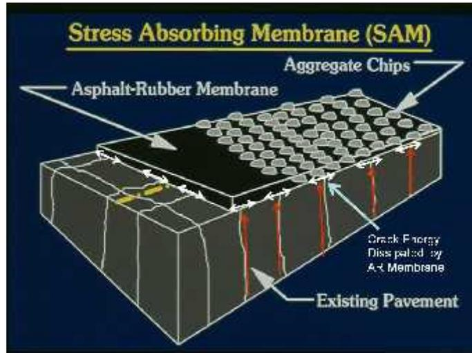
**Figure 6.** *Asphalt-rubber Stress Absorbing Membrane (SAM)*
