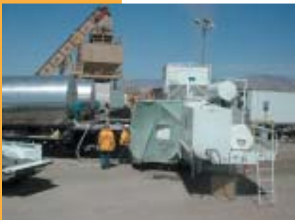
The equipment for adding crumb rubber to Hot Mix Asphalt can be set up at a typical HMA plant.
