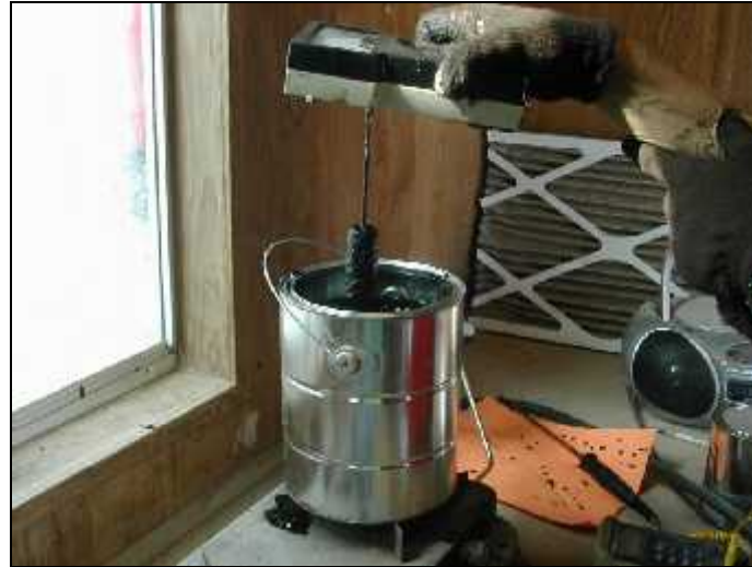
Figure 5. Typical AR binder consistency testing at 177 °C
