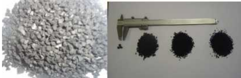
Figure 2. Photos of the crumb rubber used in this research.
