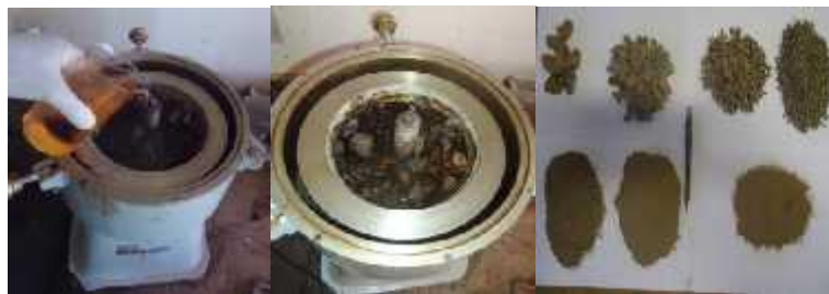
Figure 6. Extraction of asphalt binder and aggregate recovery
