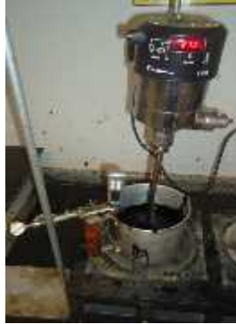
Figure 4. Mixer used to prepared the wet process asphalt rubber in laboratory
