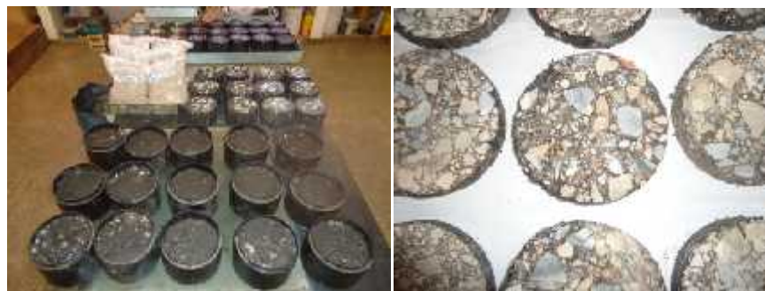
Figure 5. (a) Photos of Marshall samples; (b) Cut and polished samples.
