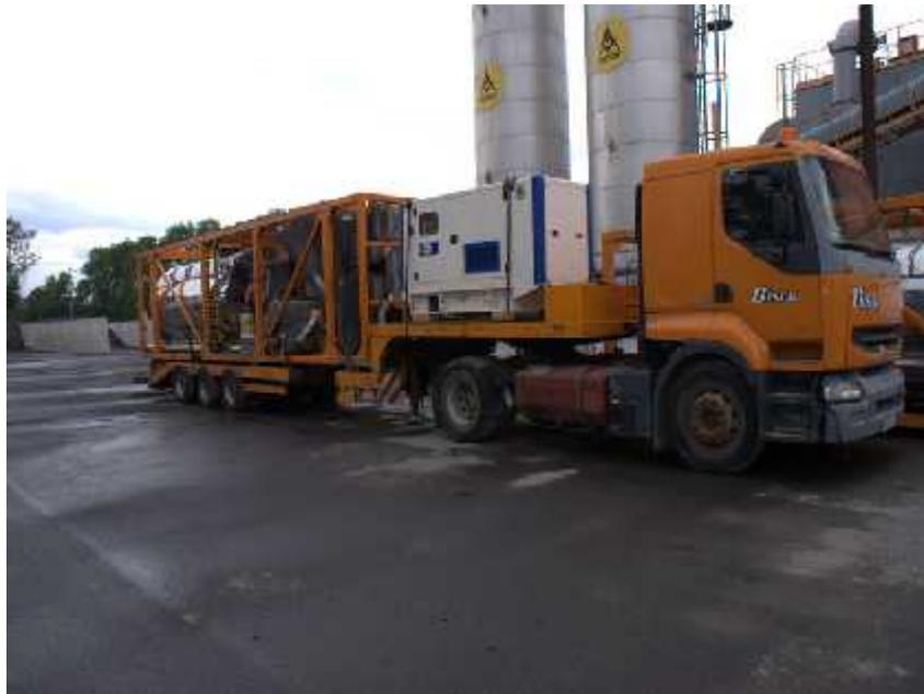
**Figure 2.** *Mobile asphalt rubber blender, Kr pice, Poland*
