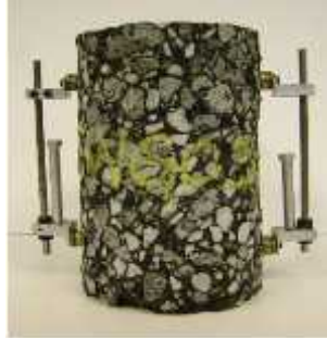
Figure 4. Typical Stockholm Swedish Gap Graded Laboratory Specimen; Sample Dimensions: 100 mm diameter and 150 mm height
