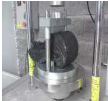
Figure 8. Indirect tension test for AR HMA
